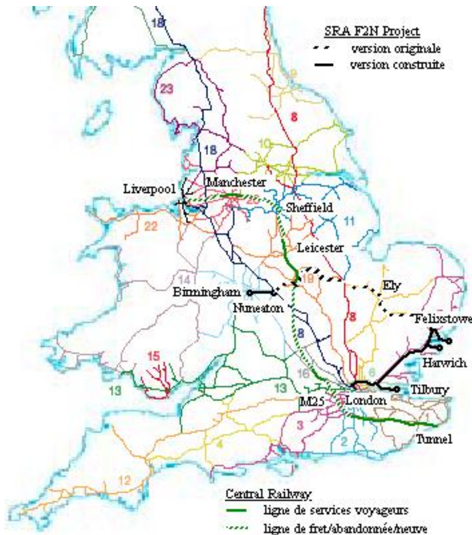
Figure 8. Projets de "Felixstowe to Nuneaton" (F2N) et de "Central Railway"
