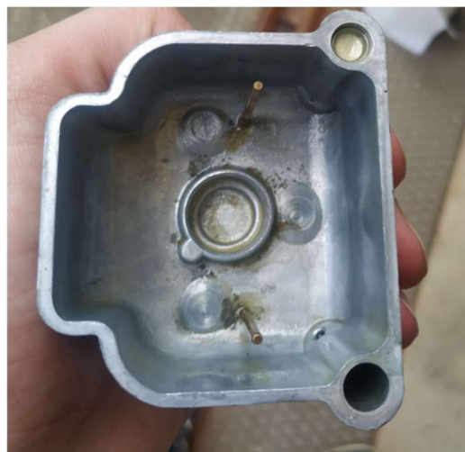
Illustration 8 Rust marks in the carburettor float bowls
