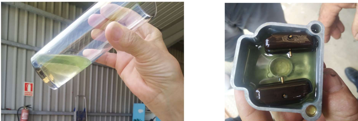
Illustration 7 Presence of water in the carburetors
