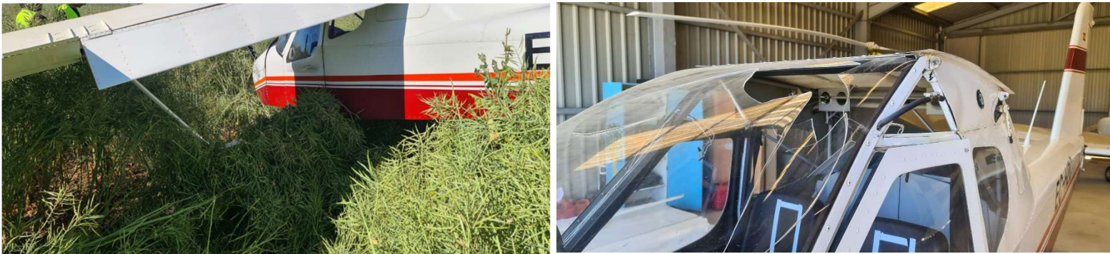
Illustration 6 Final condition of the strut and windscreen
