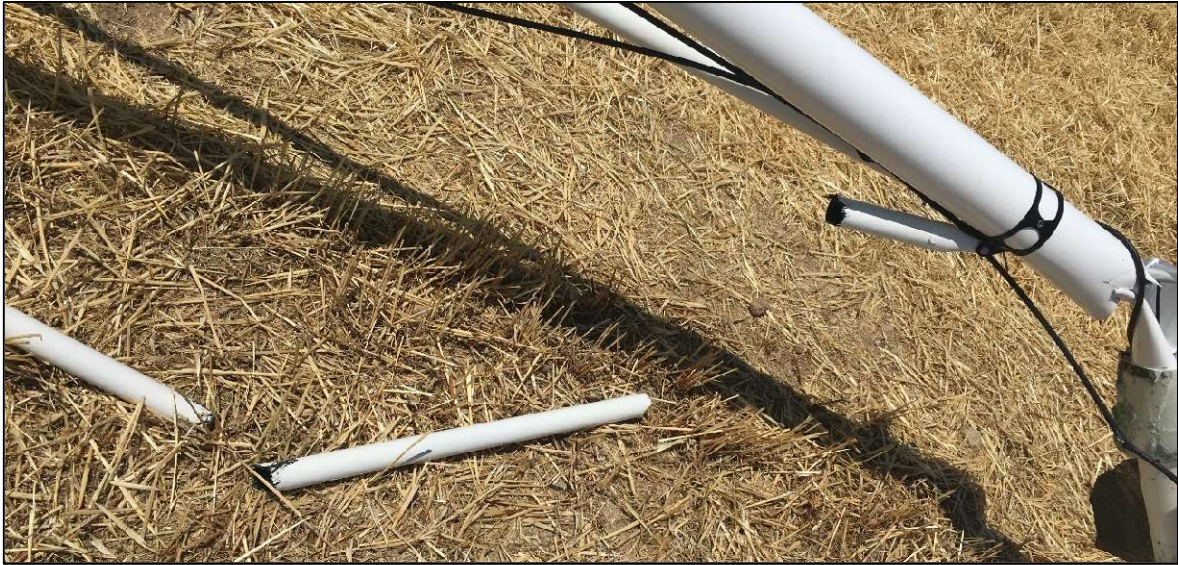
Image 10: Damaged left strut
