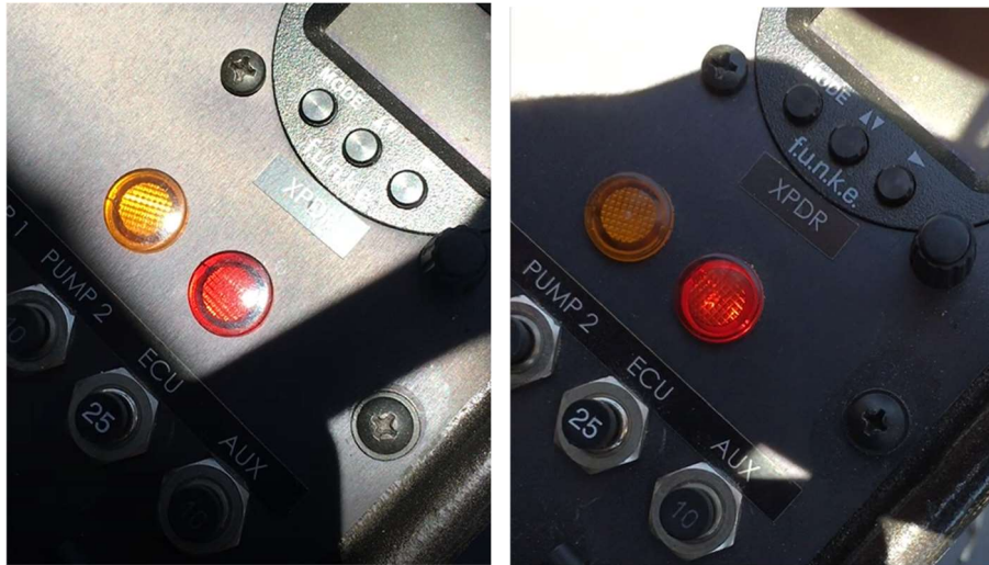
Illustration 4: impact of the sun on low battery warning light (and others)
