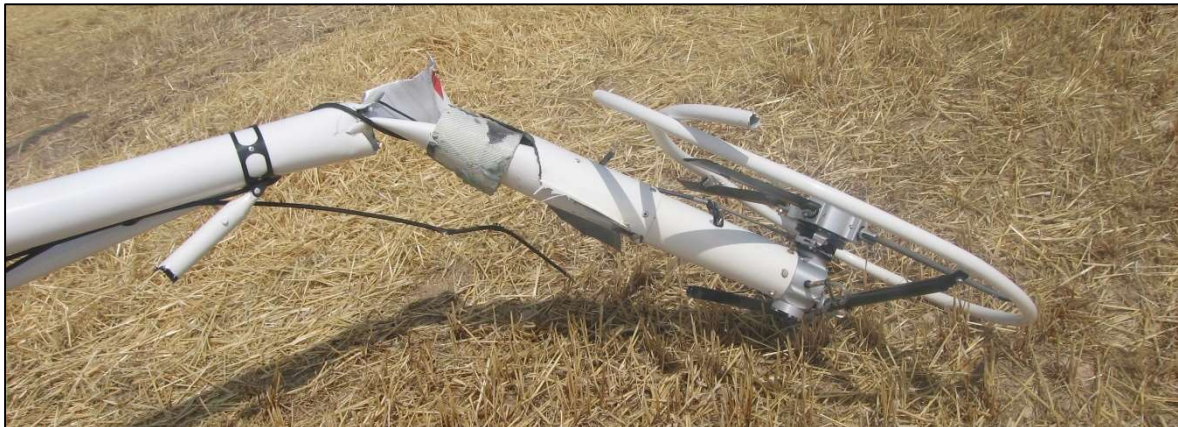
Image 9: Damage to the tail mast and anti-torque rotor
