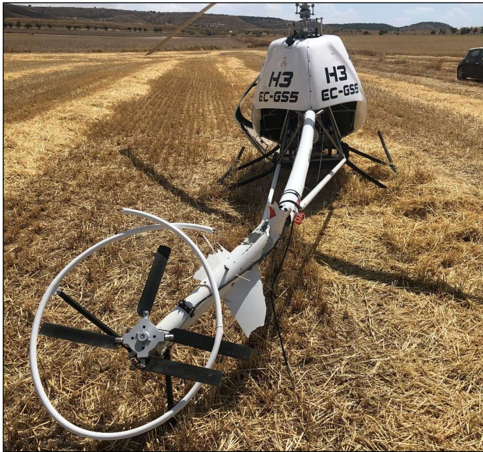
Image 13: Damage to the tail, mast struts and skids.
