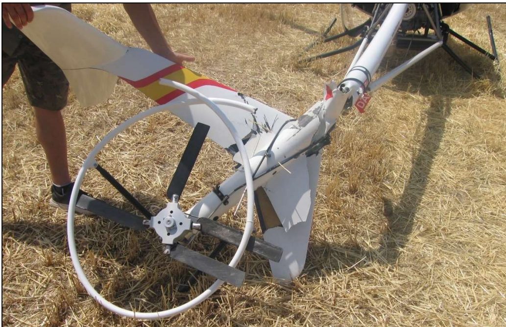
Illustration 11: Damage to the 'Shark Fin' and the anti-torque rotor
