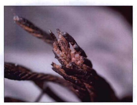
Figure 17: Close up of inner strands showing advanced corrosion
