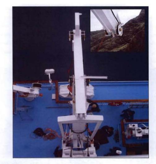
Figure 7: Lifeboat no. 9 forward davits arm showing the parted wire rope
