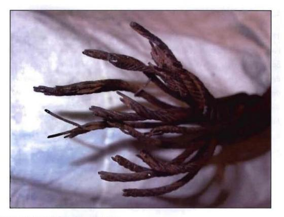
Figure 16: Inner strands of the wire rope
