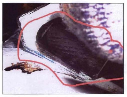
Figure 20: The wire rope open strands seen through a mirror
