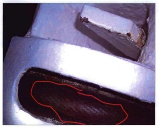
Figure 19: Wire rope strands 'opening up'
