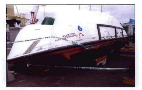
Figure 11: Extensive damage to the lifeboat tender
