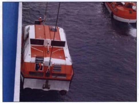
Figure 4: Lifeboat no. 9 stopped about one metre above water while the hydraulic leak was being repaired
