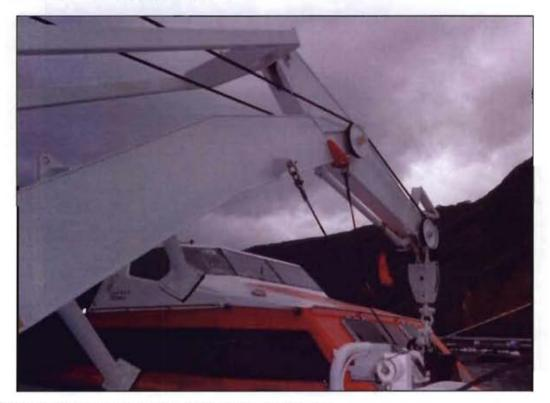
Figure 6: Block engaging with davits head (lifeboat no. 10)
