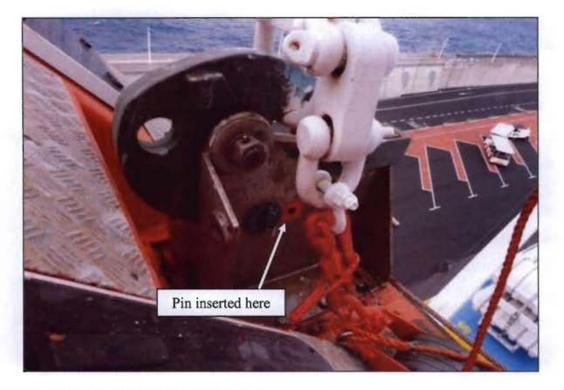
Figure 2: Locking pin arrangement as an FPD
