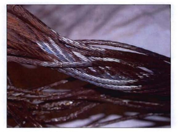
Figure 15: Evidence of residual galvanization
