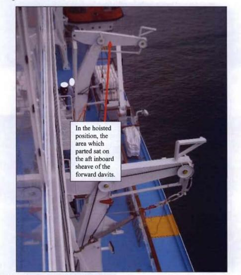
Figure 18: Davits no. 9 in the hoisted position
