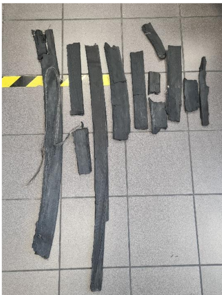
Fig. 6.- Recovered fragments of tyre tread
