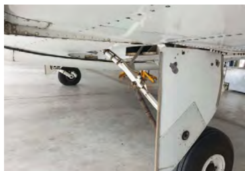
Photograph 6: Main landing gear doors
