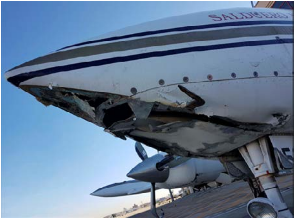
Figure 3: Close-up of the damage to the underside of the fuselage and one of the propellers
