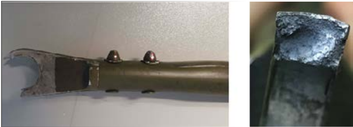
Figure 12: Close-up of the fracture on the drive tube in the front landing gear leg
