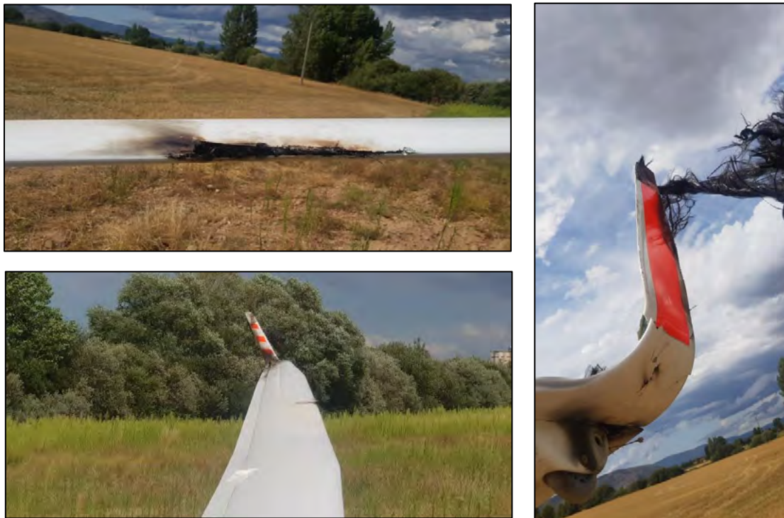
Illustration 8: Evidence of striking the cable and the resulting electric arc
