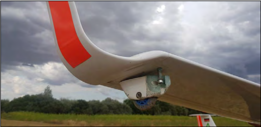
Illustration 9: Damage to the wheel at the tip of the right wing
