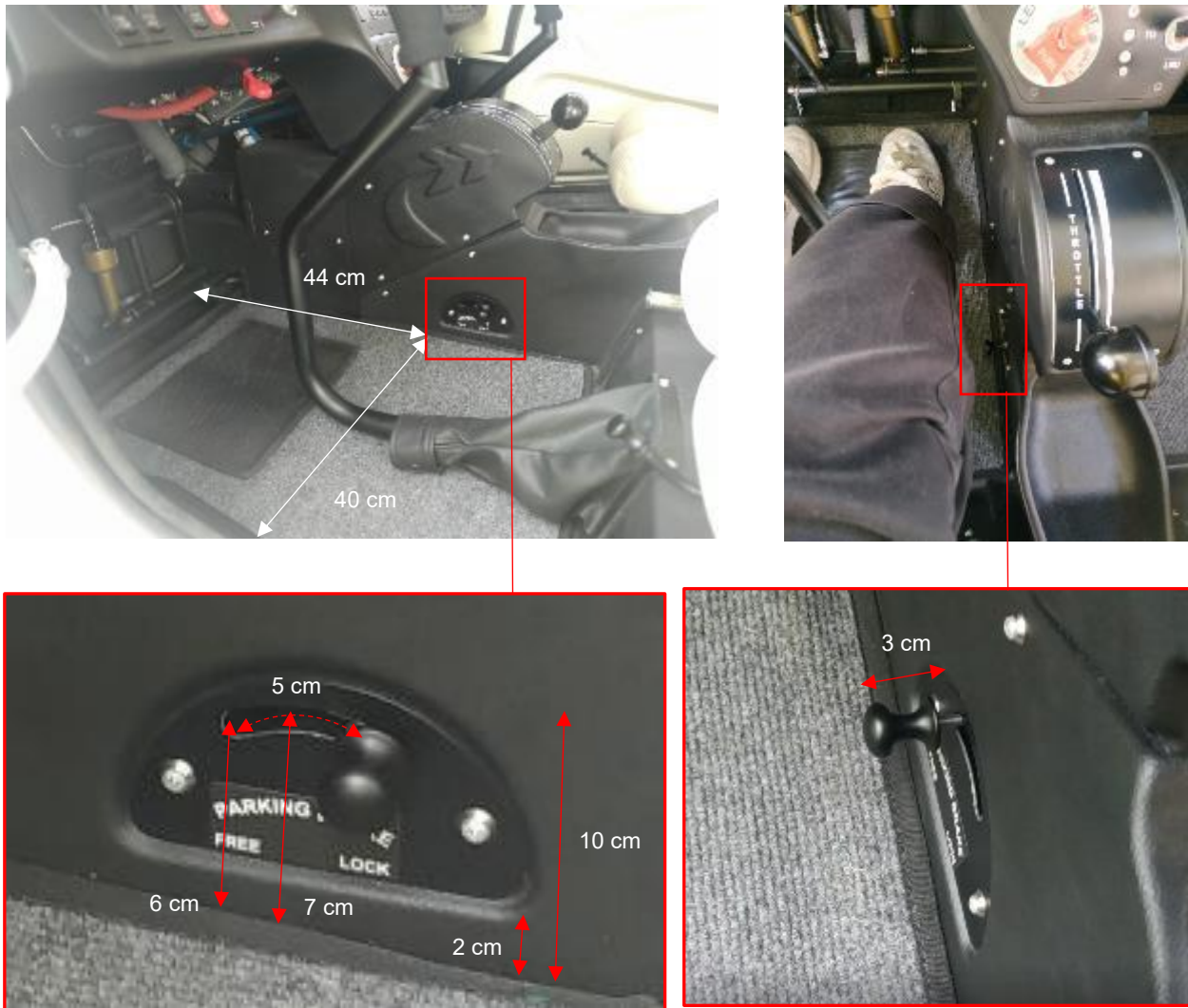
Figure 5. Position of the PARKING BRAKE lever in the cockpit
