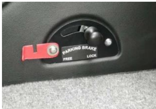
Figure 6. Catch installed by Canavia in aircraft EC-NJX
