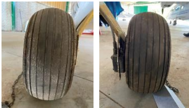
Figure 4. Marks on the right main gear tyre
