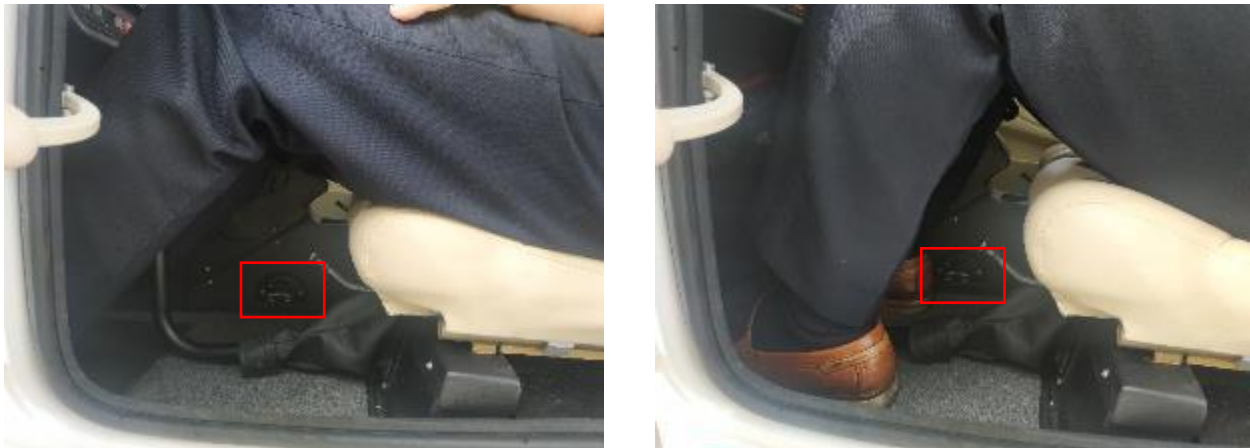
Figure 7. Position of the PARKING BRAKE lever in relation to the pilot
