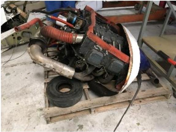
Photograph 10. Engine from the damaged aircraft
