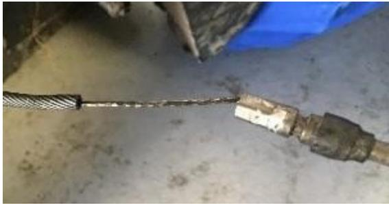
Photograph 14. Detail of the non-crimped mixture controller cable
