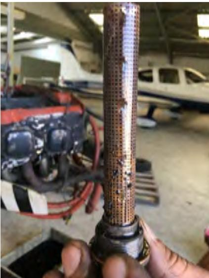
Photograph 19: Oil filter with metallic particles
