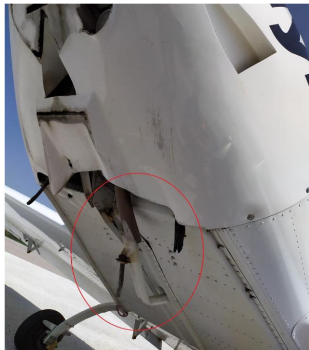
Photograph 4. Damage to nose landing gear
