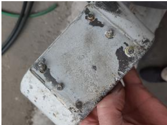
Photograph 7. Damage to lower engine cowling
