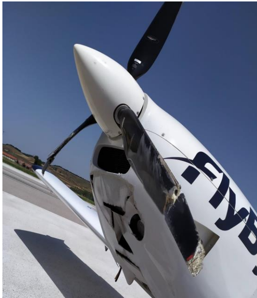
Photograph 2. Damage to the propeller
