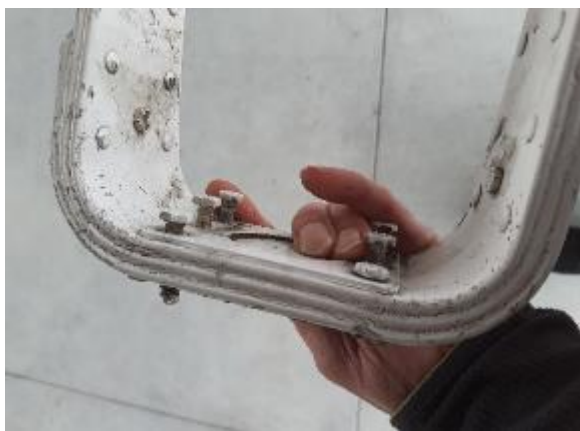
Photograph 9. Damage to lower engine cowling
