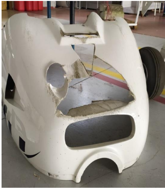
Photograph 5. Damage to lower engine cowling
