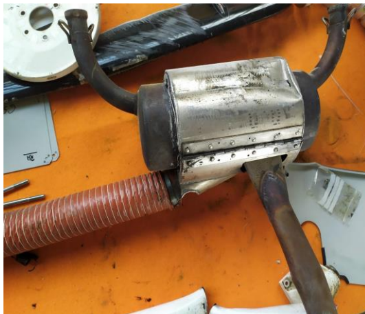
Photograph 3. Damage to the exhaust manifolds
