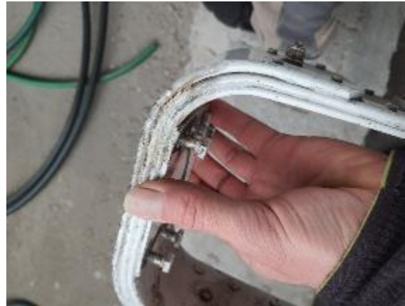
Photograph 8. Damage to lower engine cowling
