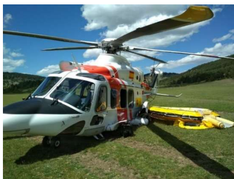
Figure 3. Status of the EC-NEH aircraft after emergency landing
