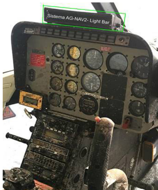
Figure 6. Instrument panel on the Bell 206B and AG-NAV light bar
