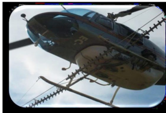
Figure 4. Photograph of a similar helicopter with the spray system installed
