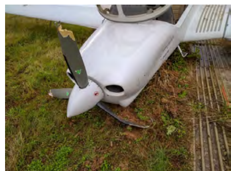
Figure 4. Damage to the propeller blades
