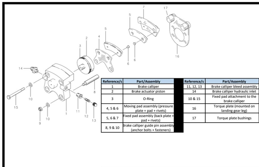
Figure 3: Diagram of the aircraft's brake.
