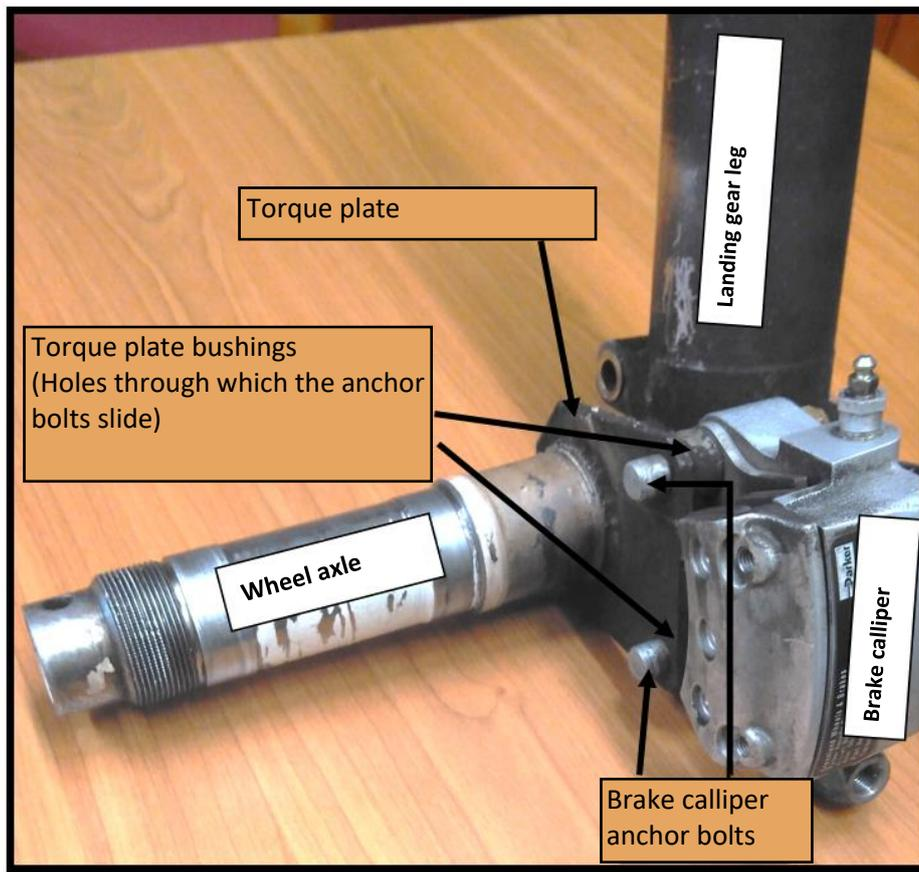
Figure 21: Brake and landing gear leg coupling.
