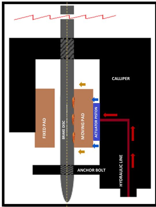
When the brake pedal is pressed, pressure is transmitted by hydraulic fluid through a line running inside the brake calliper.
