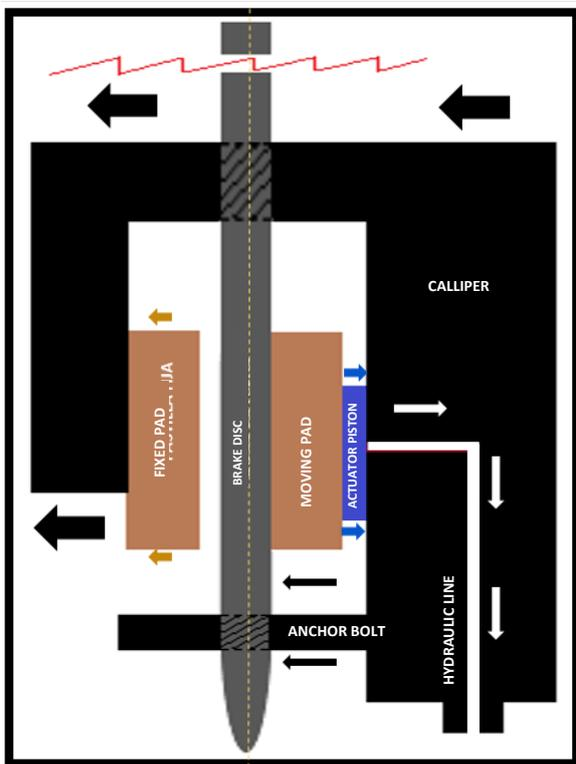
When the brake pedal is released, the hydraulic pressure is removed from the system, allowing it to return to its resting position gradually.
