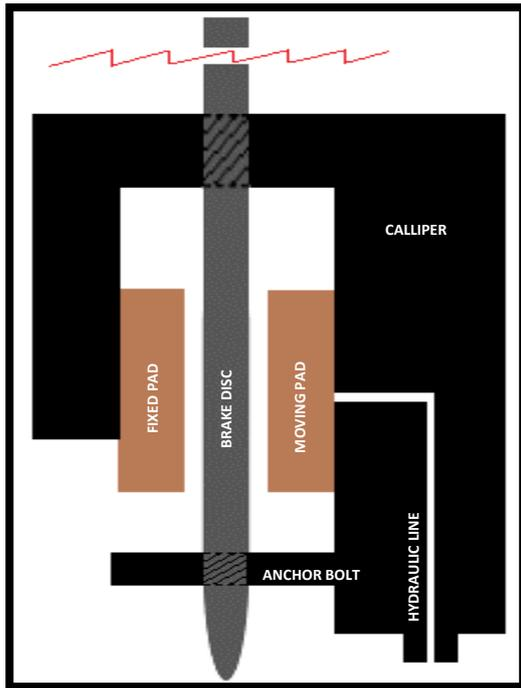
Lastly, as the actuator piston is no longer pushing the moving pad toward the disc, it moves away, freeing the disc and returning the system to its resting position (in this particular brake model, there is no retraction element as such).
