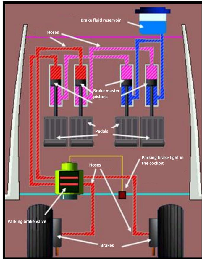
Figure 2: Diagram of the aircraft's brake system.
