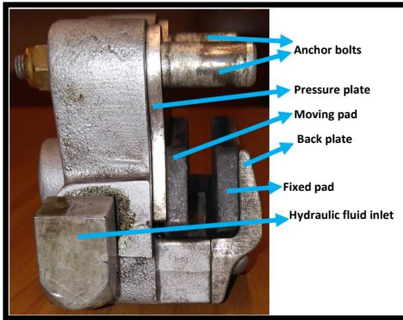
Figure 19: Brake (side view).
