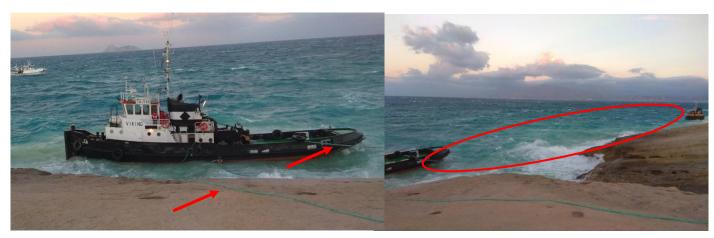
**Figure 6:** Captures during the grounding of VIKING; in the left image, the two lines indicated are the ones used for abandonment and the tow line, still attached to the dredger. In the right image the tow line is discerned floating (within red ellipse).
