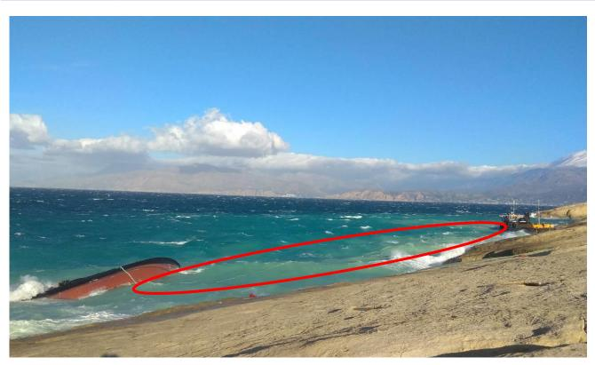
Figure 7: Capture after the sinking of VIKING. The tow line to the dredger is still floating, attached on VIKING (red ellipse).
