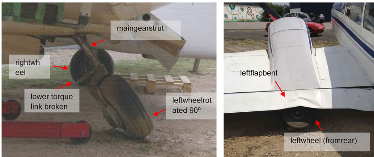
Figure 3. Gear seen from the tip (left) and trailing edge on the left wing (right)
