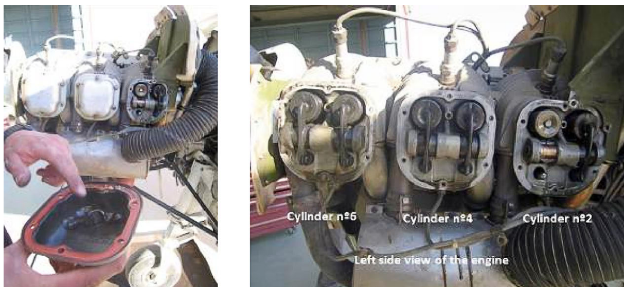
Figure 5. Disassembled covers on cylinders 2, 4 and 6 and condition of rocker arms
