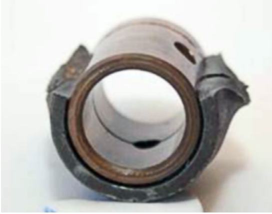
Figure 8. Misalignment of the lubrication orifices
