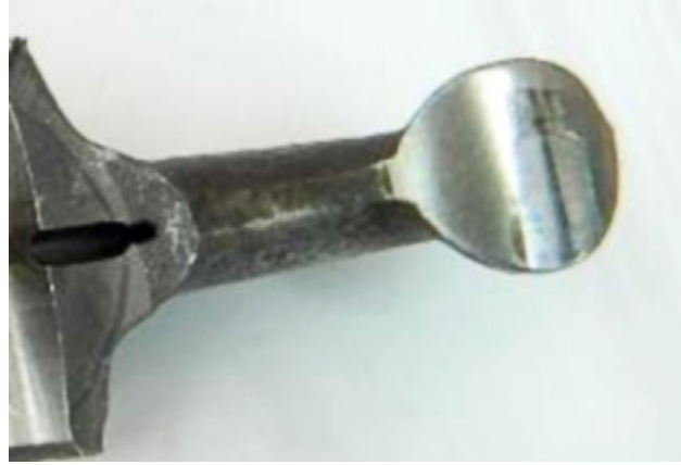
Figure 9. Flat spots on the pad of the damaged exhaust rocker arm
