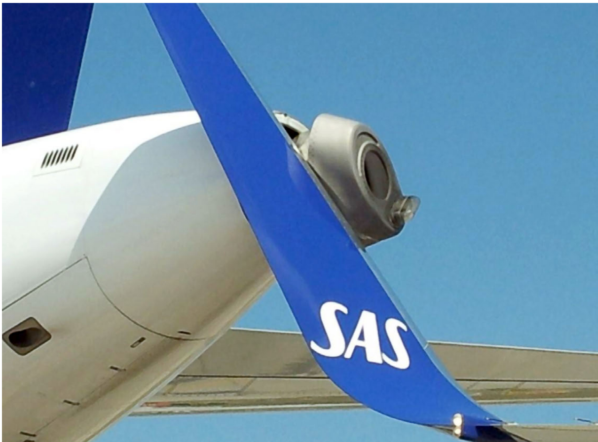
Figure 1. Photograph of the B-737's winglet caught on the A320's APU exhaust nozzle
