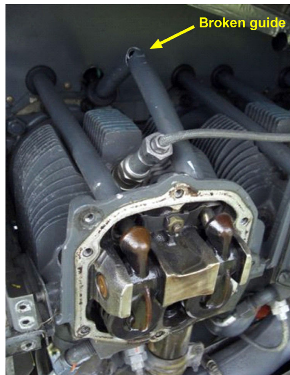
Figure 1. Photograph of broken guide
