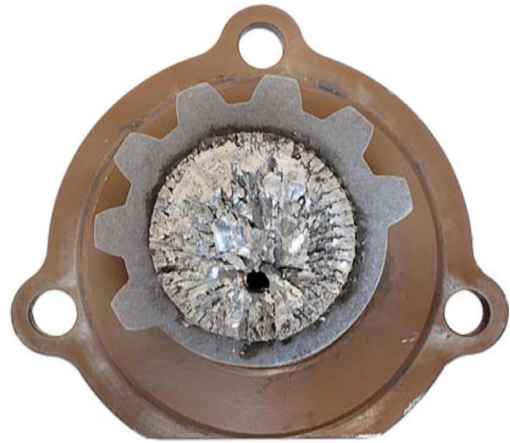
Figure 4. Cross-section of fracture
