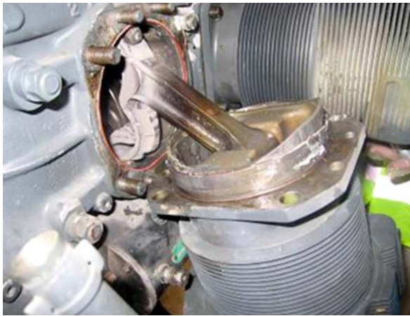
Figure 5. No. 2, cylinder, partly disassembled, showing broken connecting rod
