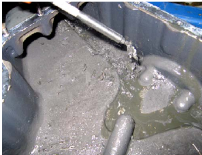
Figure 4. Metal particles and shavings in the crankcase
