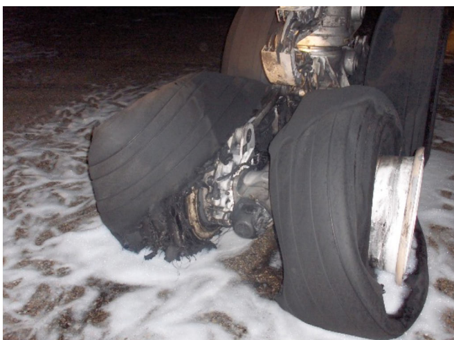
Figure 1. Condition of tires on wheels 5 and 6
