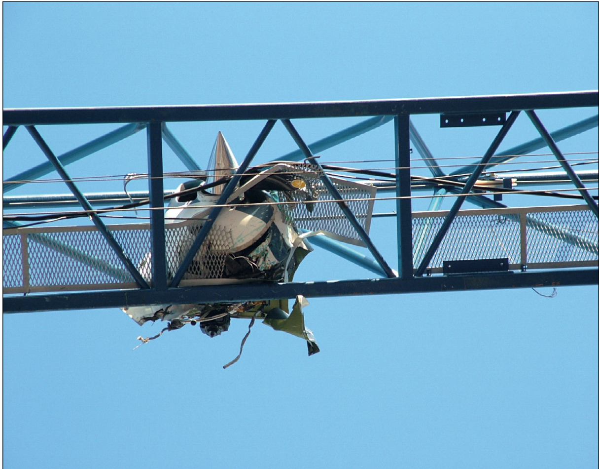
Figure 1.4. Photo of the powerplant stuck in the crane structure
