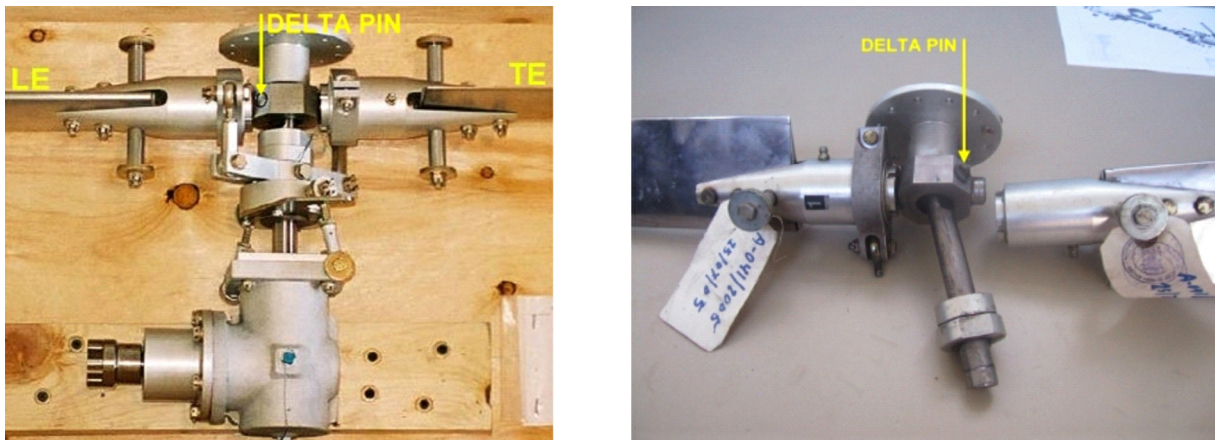
Figure 7. Spindle assembly according to CHR's Compliance Procedure (left); asfound assemble of the tail rotor (right)
