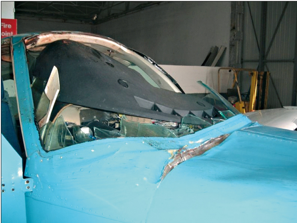
Figure 1. Damages of the bird impact with aircraft
