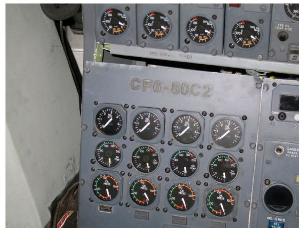
Figure 3. Flight Engineer's panel
