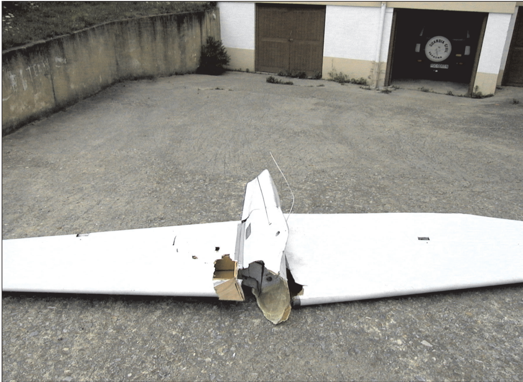
Photo B-1. Stabilizers wreckage
