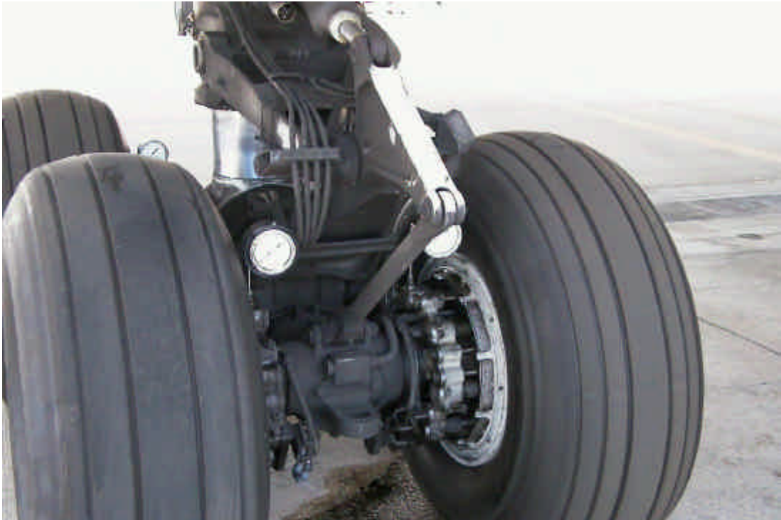
Gauges installed on the brakes of TF-ATH
