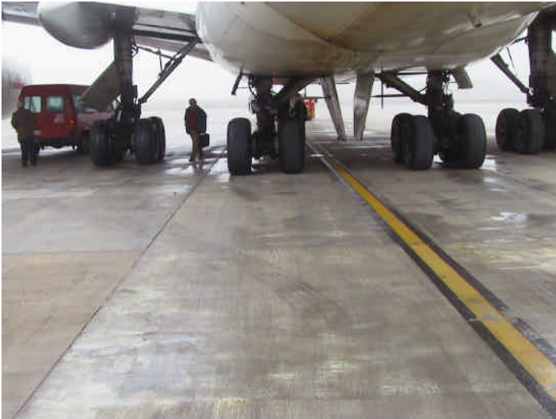
Ground marks during the taxi tests (continuous and lightly marked)
