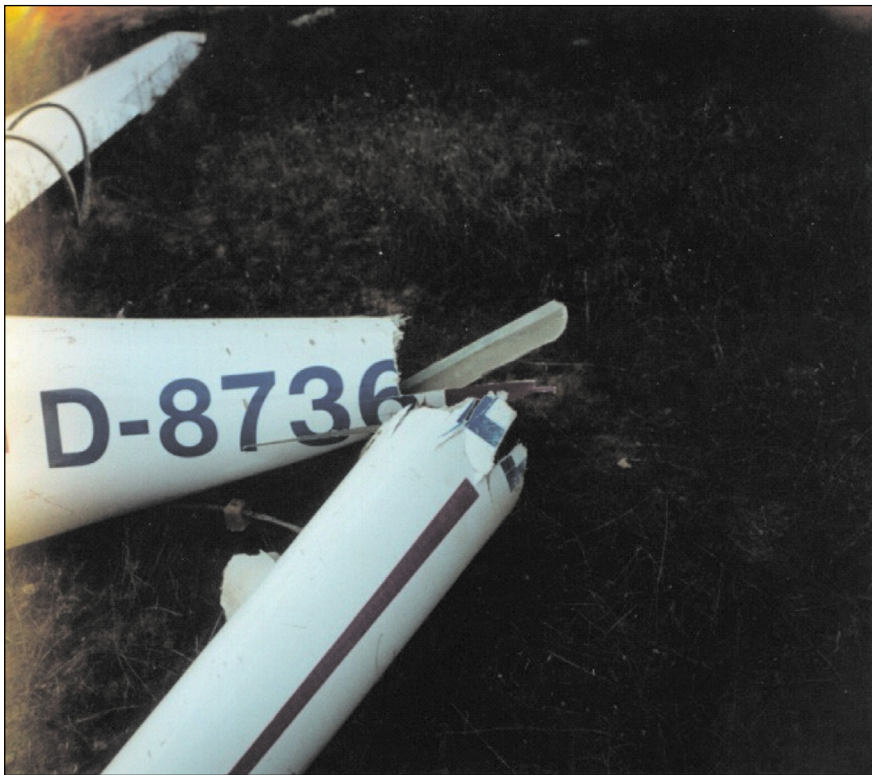
Figure 4. Detail of fuselage breakage
