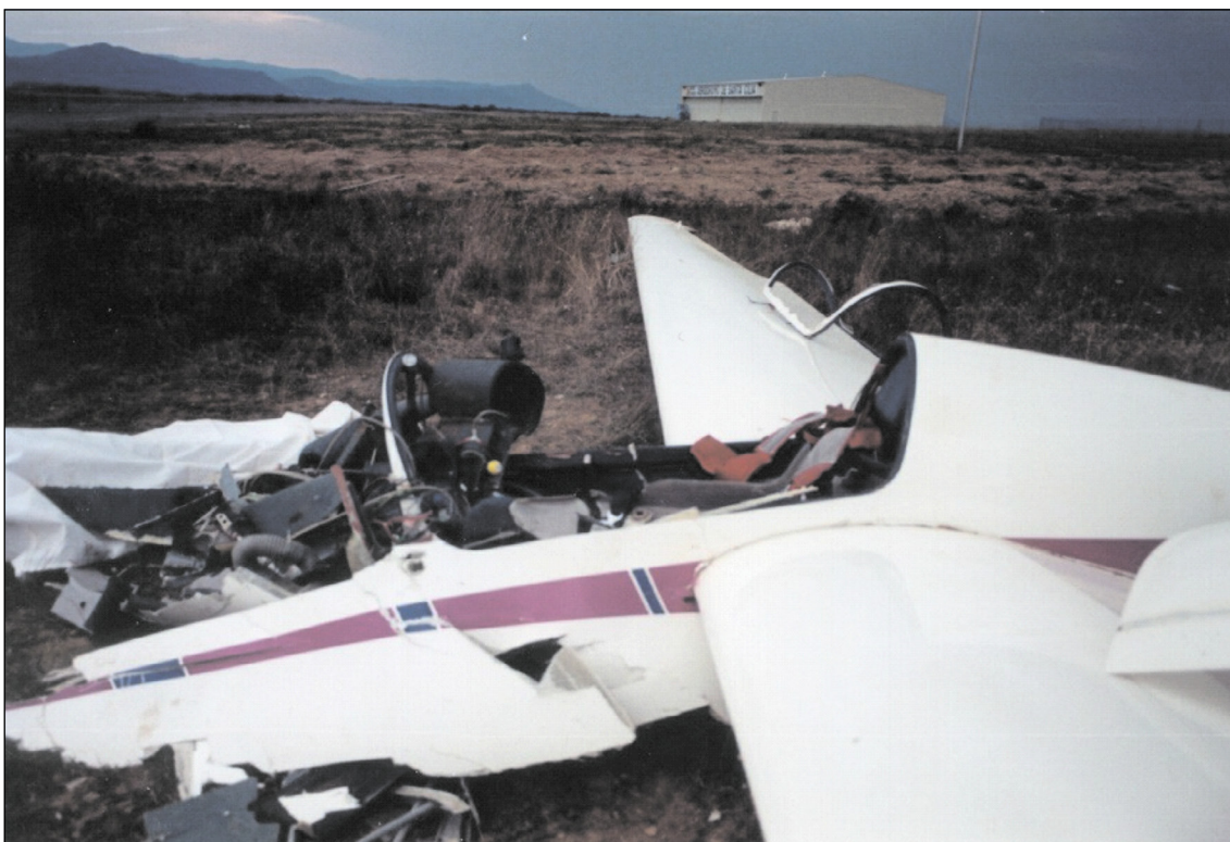
Figure 5. Front fuselage and cockpit wreckage
