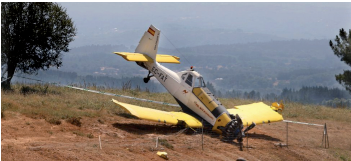
Fig. 3. EC-FAT. Damage to the left wing
